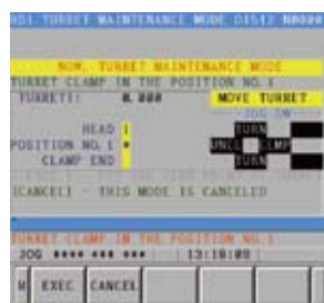
Turret Maintenance Used to adjust the turret zero point.
